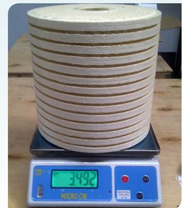
Dirty and clean CJC™ Filter Inserts. The dirty insert is 12.17 kg heavier! (after being drained)
