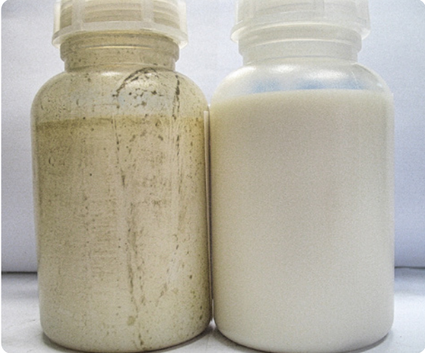
Lubricant samples – left without, right with depth filtration
