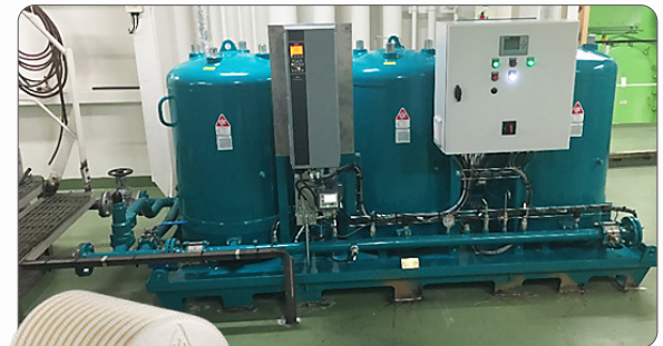
CJC® Oil-Care System 3x427/81 and integrated CJC® Fine Filter Insert LOX – specially developed for lubricating oil care on 2-stroke diesel engines
