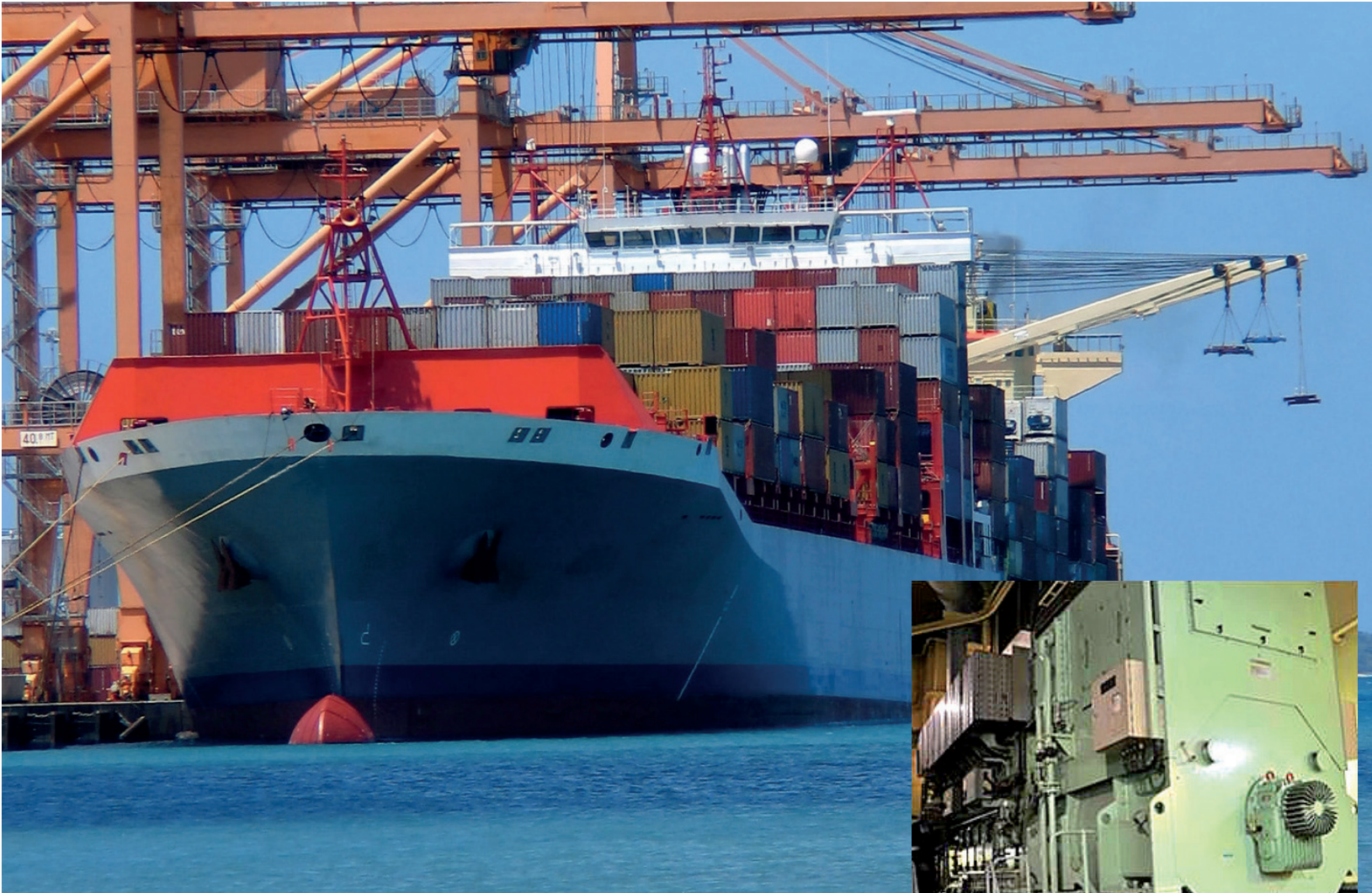
Container Vessel, 4,200 TEU Engines MaK 6M332, 2,880 kW
